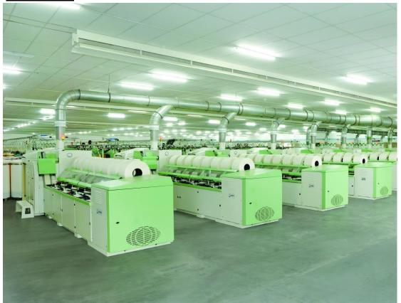
Comber LK64 Z with technological speeds of upto 500 NPM, incorporated with (MCDP Plus) is designed to produce upto 1.7 tons/day of combed sliver. This technology, combined with specially profiled, light weight aluminium alloy Nippers and reduced number of moving parts, assists high speeds and productivity
